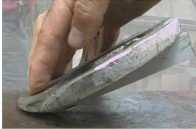
▲FIGURE 10.10 Hand forged heart-bar support shoe. The toe of the shoe has been rolled and the ease of break-over is being demonstrated. Triangular shaped rails have been bolted to the underside of the shoe to provide heel elevation (Shoe forged by Craig Jones of Brisbane, Queensland).
